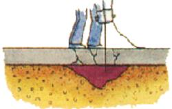
Drill concrete floor along all expansion joints and cracks, and treat soil thereunder
