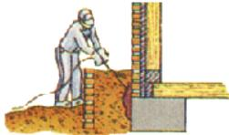
Use rod injection to treat soil along and around the external perimeter area of the building
